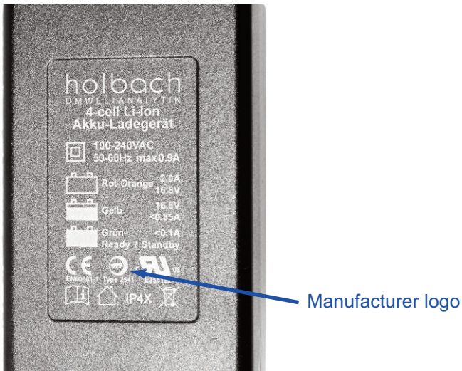
Figure 14 The rear of the charger contains the status colors, certification mark and manufacturer logo
