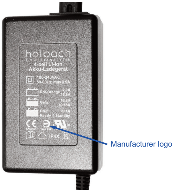
Figure 11 Rear of the charger containing the status colors, the certification mark and the manufacturer logo
