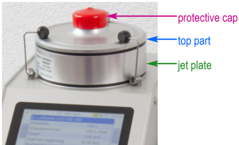
Figure 38 The air sampler's components
