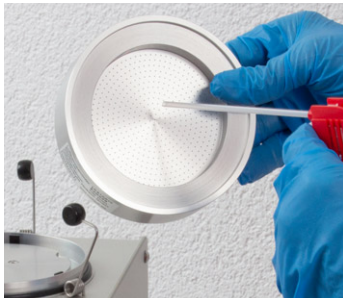
Figure 46 Blow-dry the jet plate
